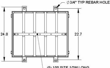
(5) 100 SIZE 1/2M LONG CENTER BOLT LOCK (NOT STARFIX) GRATES FIT IN TOP AND SECURE TO CROSS MEMBER
